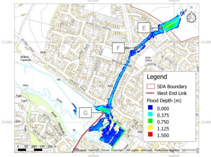
**Figure 4 – Hailey Road drain flood extents**
