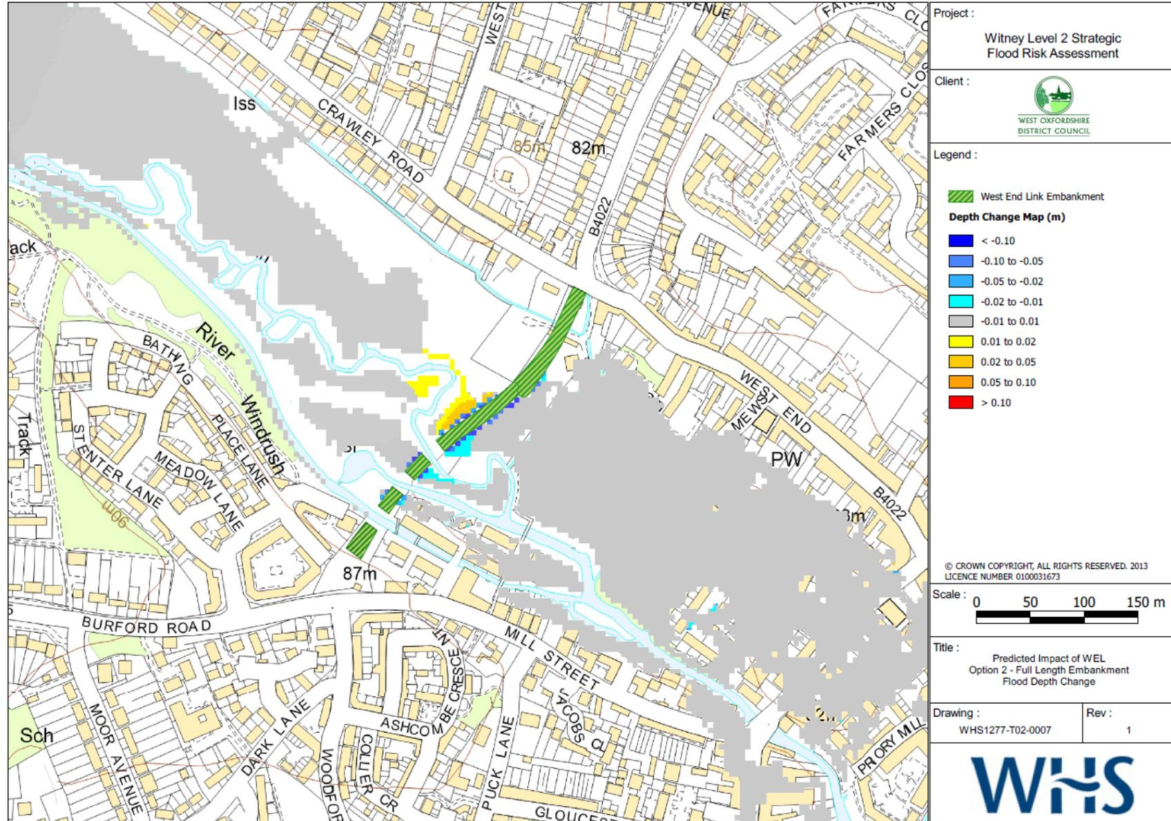
Figure 6 – Impact of Option 2 on Flood Depths
