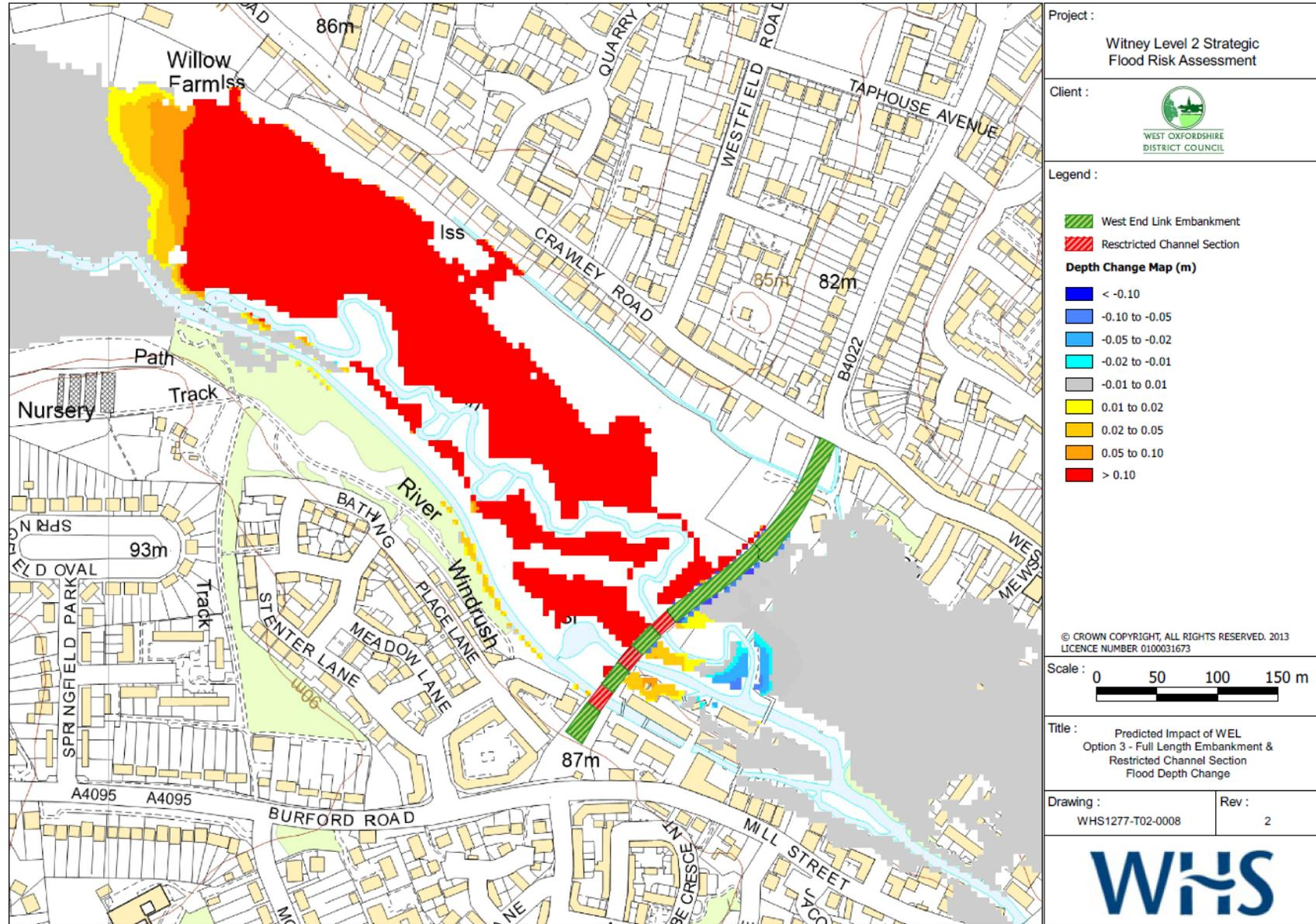
Figure 7 – Impact of Option 3 on Flood Depths
