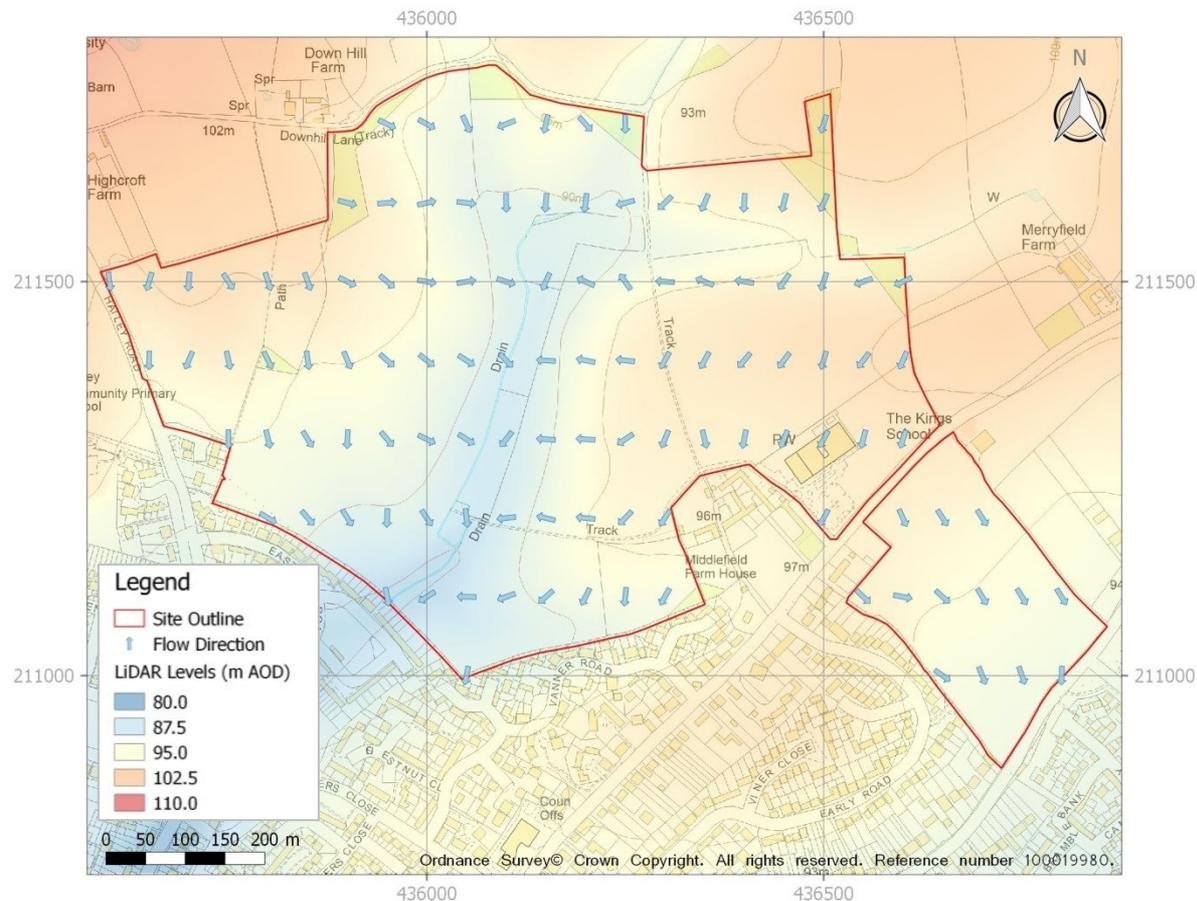
Figure 2 – Topography based on LiDAR aerial survey data
