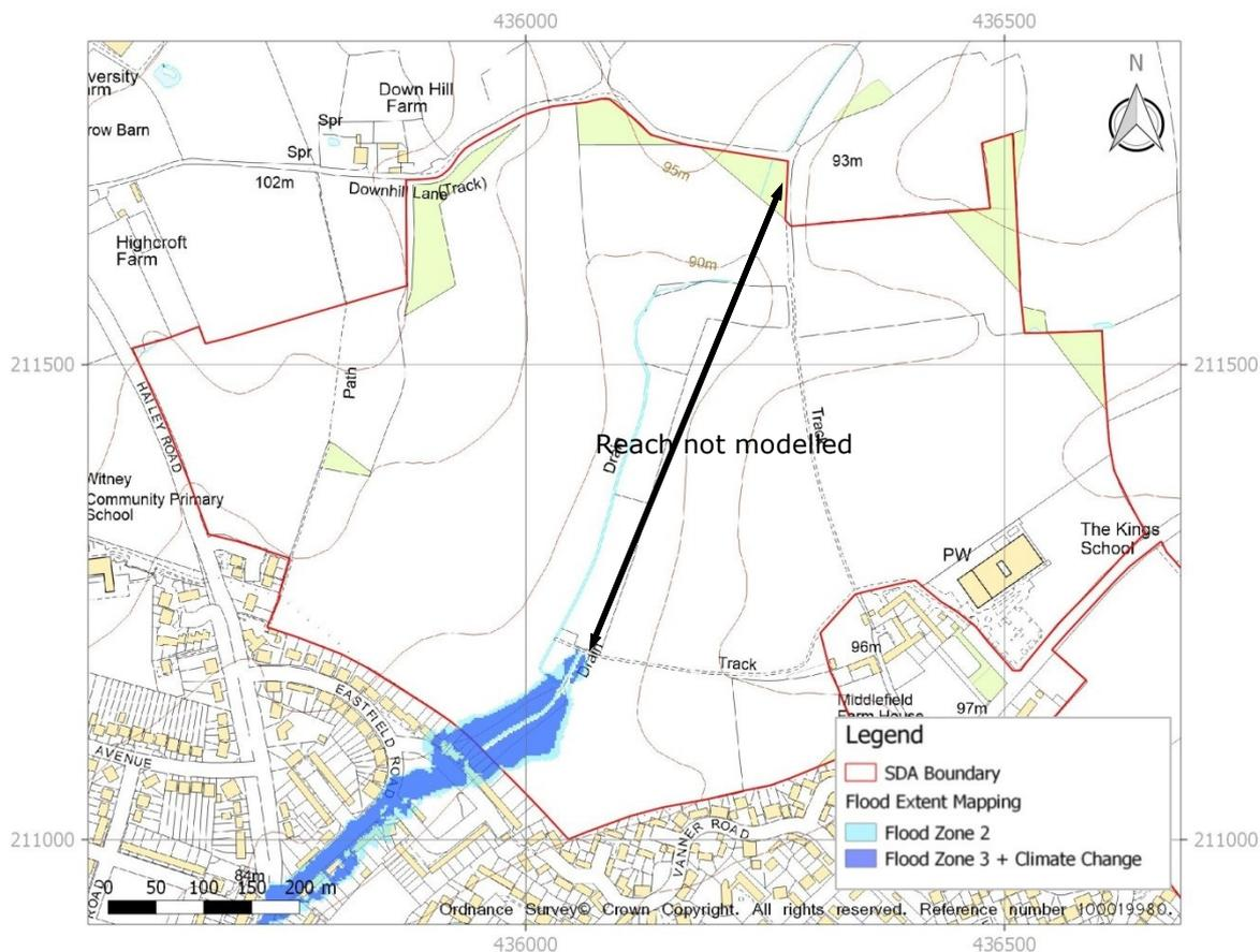
Figure 3 – Existing model extents of Hailey Road drain
