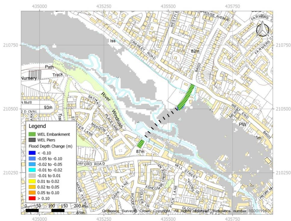
**Figure 8 – Flood Depth Change as a result of the WEL Option 1 (viaduct on piers)**
