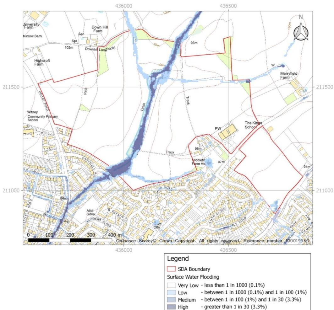
Figure 6 – Pluvial Flood Map
