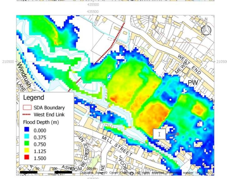
Figure 5 - Windrush flood extents, focused on proposed West End Link
