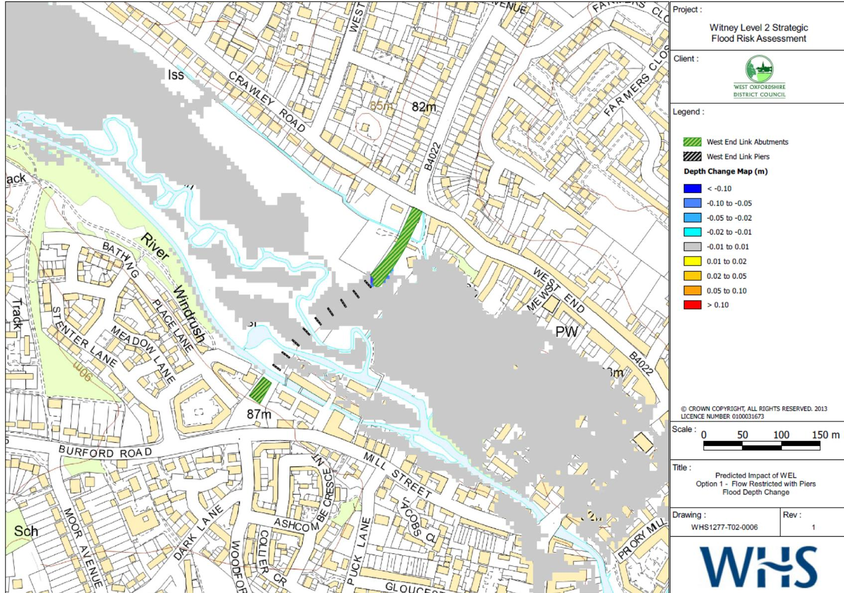
Figure 5 – Impact of Option 1 on Flood Depths
