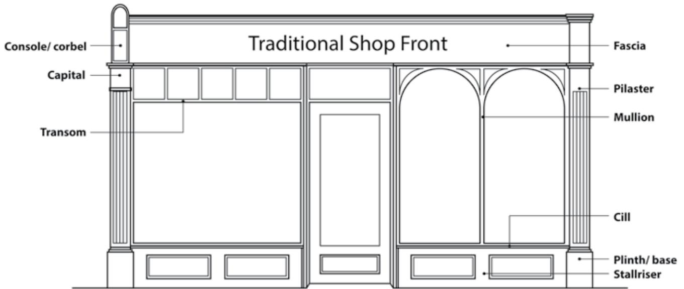
Fig. 5 The components of a traditional shop front
