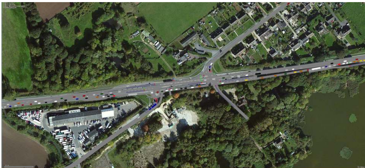
Figure 6– Blocking back through Cassington Road signals in the westbound direction
