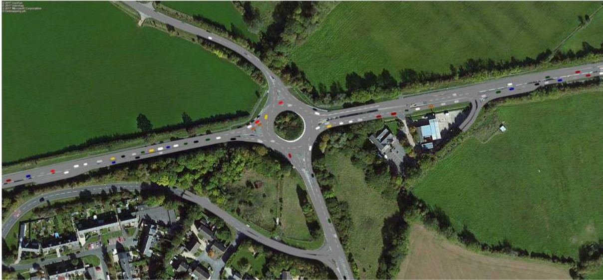
Figure 7 – PM peak queues on both A40 east and west approaches to the Lower Road roundabout
