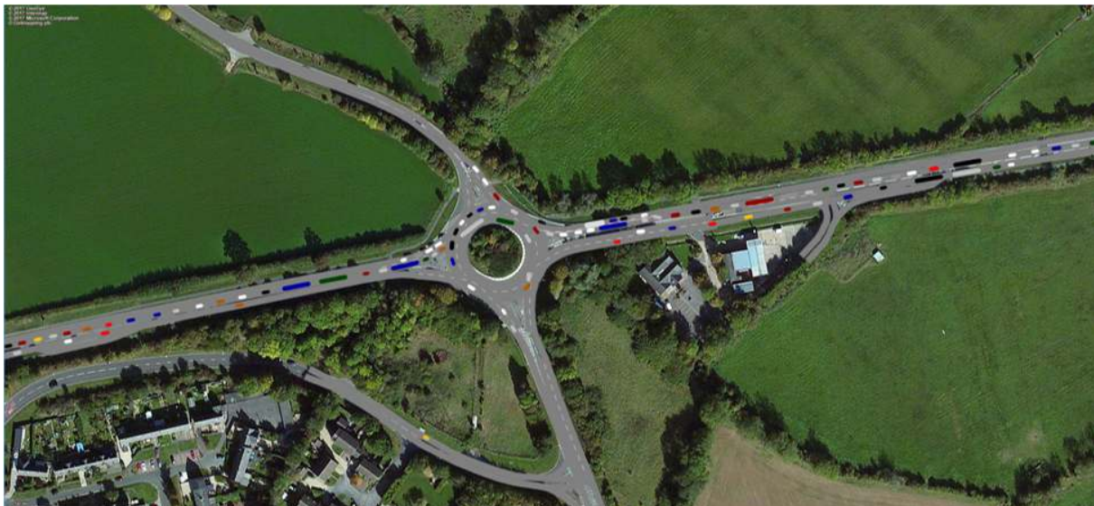
Figure 4- AM peak period blocking back on the A40 through the Lower Road roundabout in the eastbound direction
