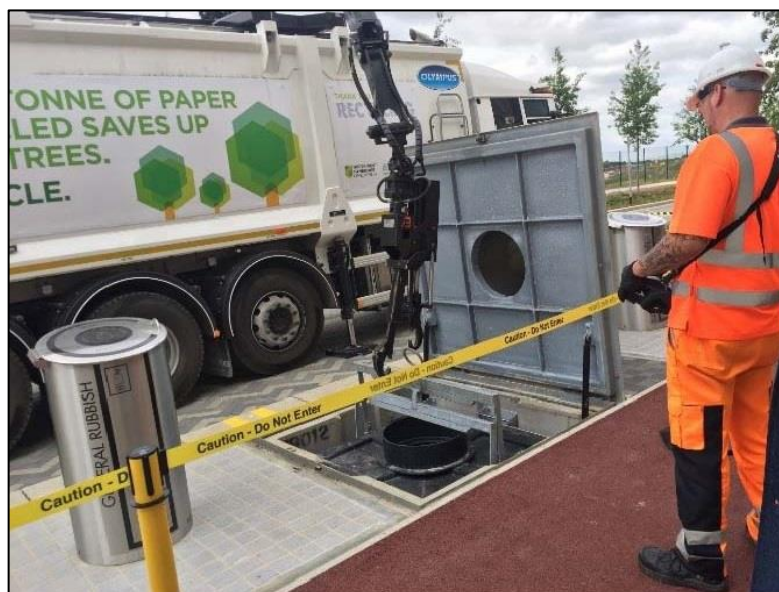
Figure 2: Waste collection operative emptying a URS unit using a hydraulic mechanical lifting arm. The process can be completed by one individual and provides a safer/less physically demanding approach for waste collection.
