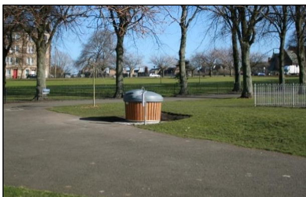
Figure 4: Underground silo bins in Princess Street Park (left) and Harrison Park (Right), Edinburgh. 16 underground bins were used to replace over 200 on-street litter bins. In addition to environmental and financial benefits, the large waste storage capacity reduces the chance overflowing and therefore keeps the collection area tidy despite heavy footfall.
